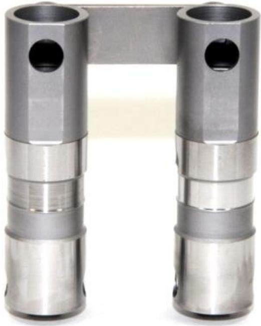
Street series lifters are used for cam profiles designed for mild street use or cams that are cataloged by GM, Ford, or Chrysler and designed for a .700" wheel. Morel does not recommend using them on anything more than .375" lobe lift and .050" duration no over 245 degrees. We recommend 1 full turn of preload. This is a slow leak down lifter. Available for all domestic production V-8 engines. Max spring pressure 150/400#
