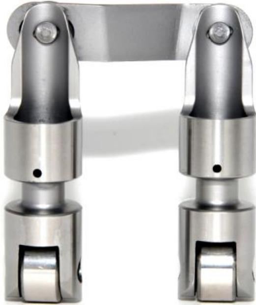
Pro Series lifters are based on the industry standard body design with a cutaway oil band. This lifter is recommended for use in performance drag race and circle track engines. This lifter should not be used in applications that require extended idling times. This lifter does not have pressure fed oiling. It does feature a full .750" wheel. Available for Chevy, Chrysler, and Ford production V-8 engines. Recommended spring rates of 250/600#.
