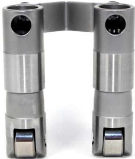
The Pro Series hydraulic roller revolutionized the hydraulic roller cam business in 2003. This lifter is made from 8620 tool steel and features a .750" wheel. With the ability to use springs up to 220#/525# this lifter will allow an engine to rpm well past the 6500 rpm range and not nose over. The lifter cannot be used with oil weight heavier than 15W40. Available for Chevy, Chrysler, and Ford production V-8 engines. We recommend 1 full turn of preload. This is a slow leak down lifter.
