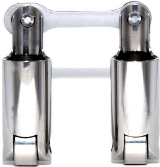
Design for Top Alcohol Hemi Based Blown engine applications. This is for all engine blocks set up for .903" lifter diameter with 2" lifter bore spacing. Machined from tool steel. Designed for extreme pressure loads.
